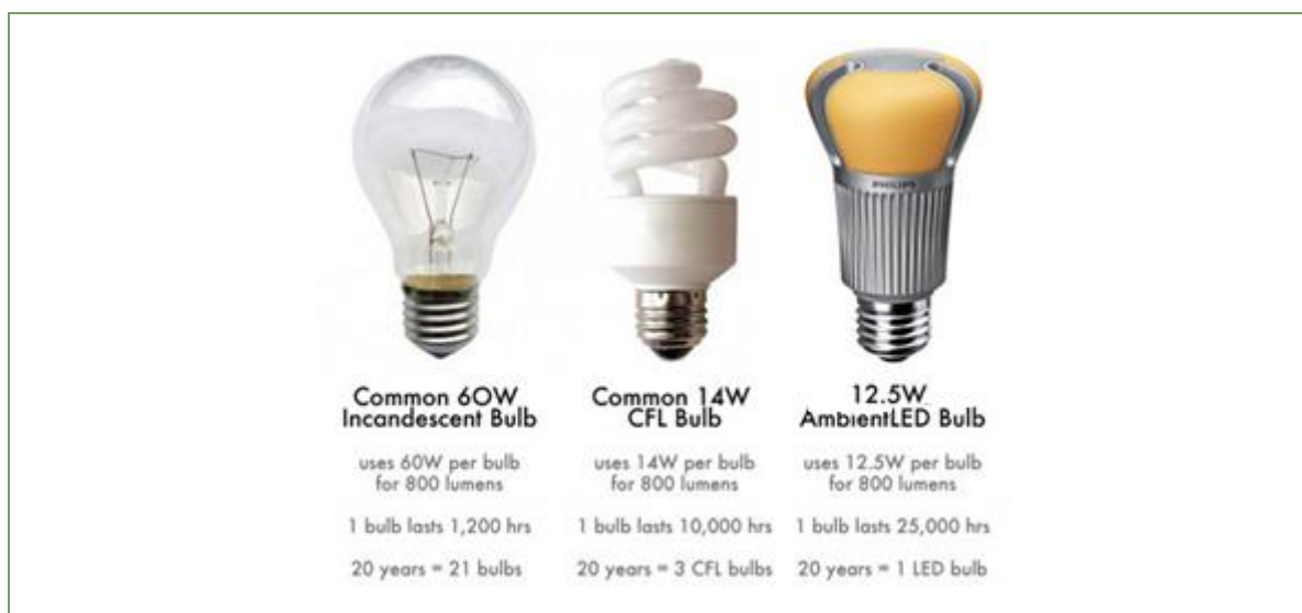
Figure 3-2. Comparison of incandescent, CFL, and LED electricity use and lifetime 30
